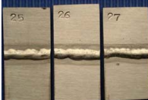
Hastelloy alloy C-22 w/ INCO-WELD Filler Metal 686CPT
